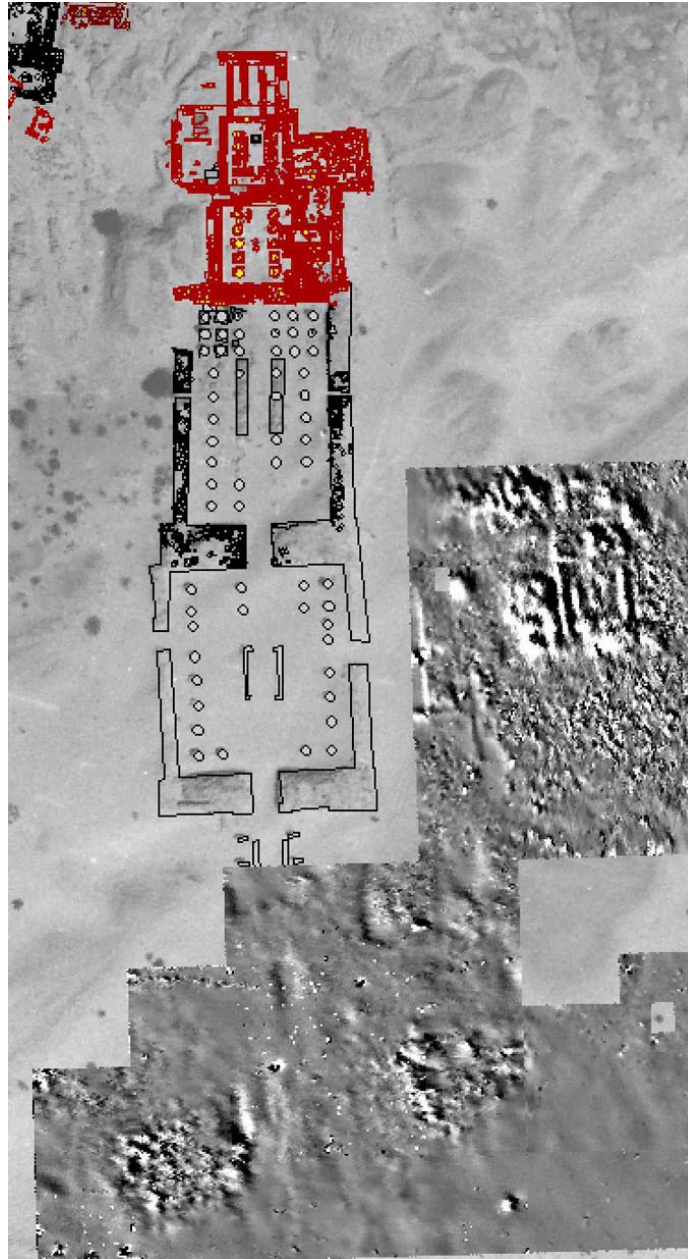
Fig. 1. Magnetic image generated in 2006 showing B 500 with previously unknown structures (then buried and not visible from the surface): at right (NE): B 1700; below: the mammisi temple and kiosk (B 560-561) on right side of avenue leading into B 500, and opposite it: a still unexcavated temple (B 570). (Geophysics: Meg Watters, T. Goldman, R. Wutzler, and Moh. Abdul Wahab).
